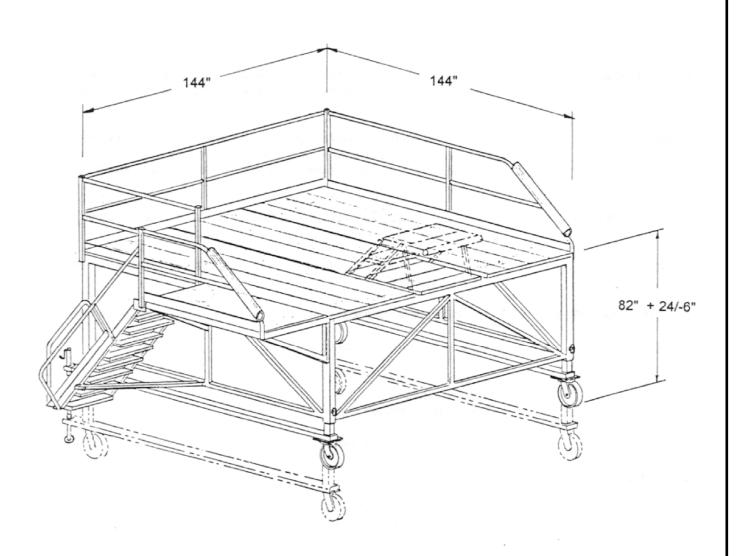
WIDE BODY AIRCRAFT FORWARD CARGO STAND Assembly -01 for A-300 Shown Assembly -03 for DC-10 MD-11 A-330
