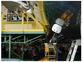
Overall Length – 252" Overall Width – 210" Overall Height – 127" Nominal work deck size 192" x 240" Working level height adjustable 84" to 144" Pneumatic Powered Screwjack Height Adjustment
