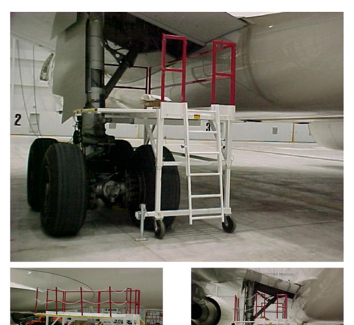
•Adjustable Ht.,Removable Guardrails, and Sliders allow configuration to Multiple Aircraft (747, 777, 767, A330, A310, A300)
