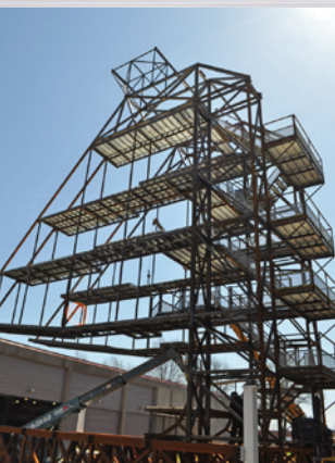
B777 tail dock – This docking system was preassembled for customer approval before shipment and was installed at the customer site by our team of technicians.
